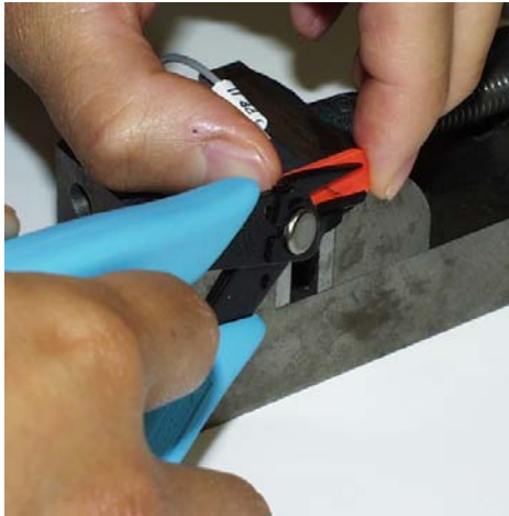
Figure 73 Cutting Wires Flush with Gauge
