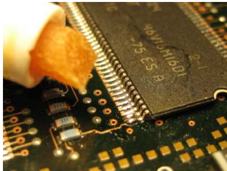
Figure 45 Fluxing of the Target Points
