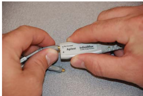
Figure 8 Properly Pulling the Probe Head Straight Out
