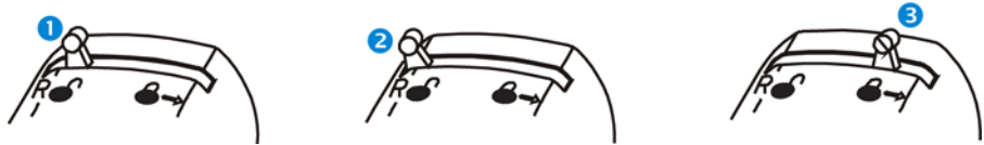
Figure 11 Properly Connecting a Probe to the Oscilloscope
