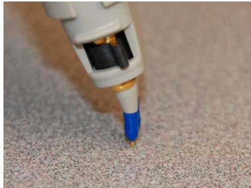
Figure 35 Proper Vertical Orientation of the Blue Tips
