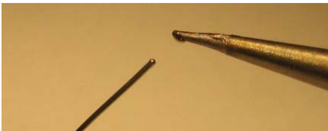
Figure 46 Small Amount of Solder Added to Soldering Iron Tip
